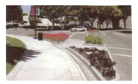
The above illustrations shows how a curb extension can reduce the turning radius and vehicle turning speed.
